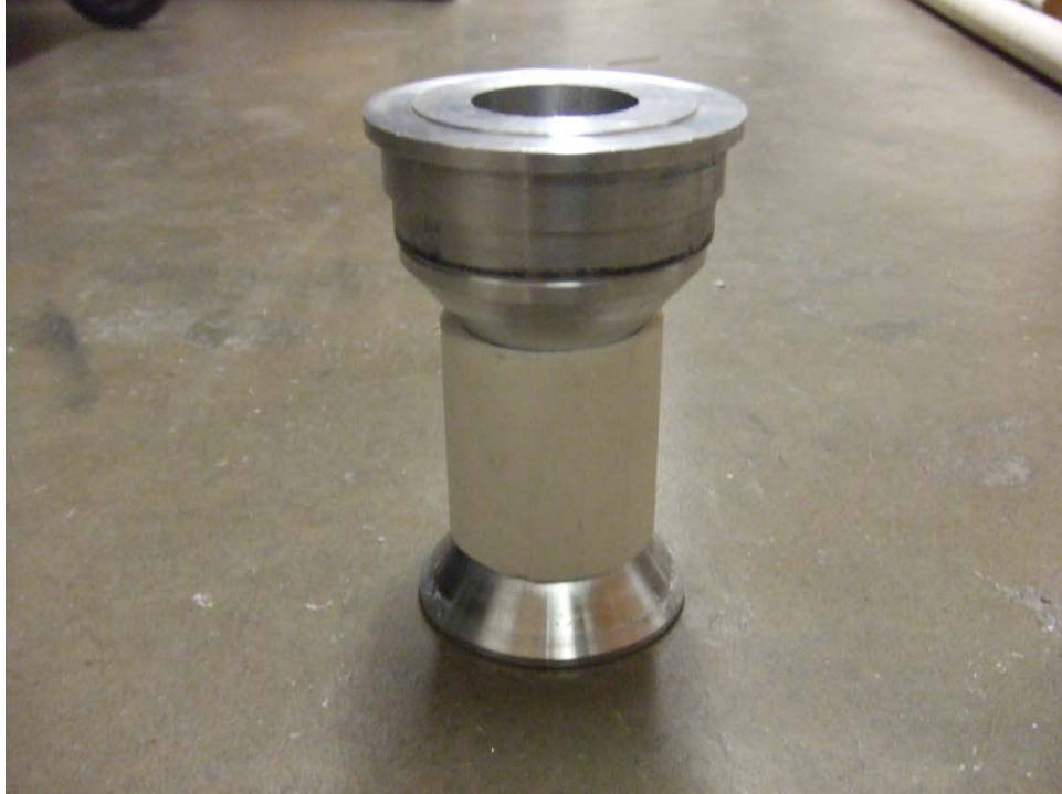
Figure 7.2.21: PVC section in jig before pressing.
