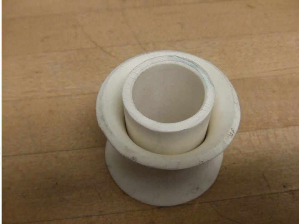
Figure 7.2.26: 1" schedule 40 PVC fits inside pressed hinge piece with enough room for rotation.
