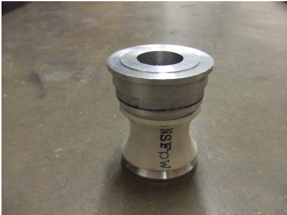
Figure 7.2.22: PVC section in jig after pressing.
