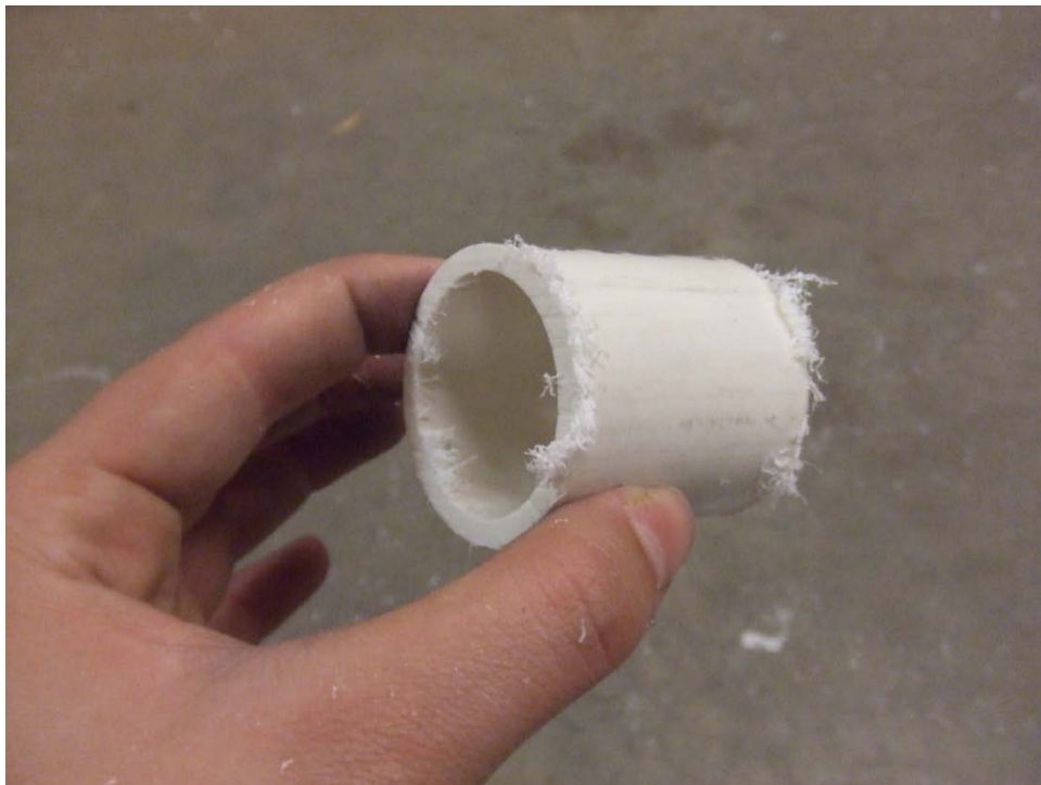
Figure 7.2.15: Short section of PVC tube cut on band saw.
