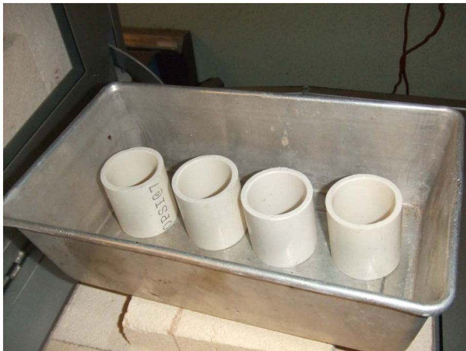
Figure 7.2.17: PVC sections being loaded into the oven in groups of four.
