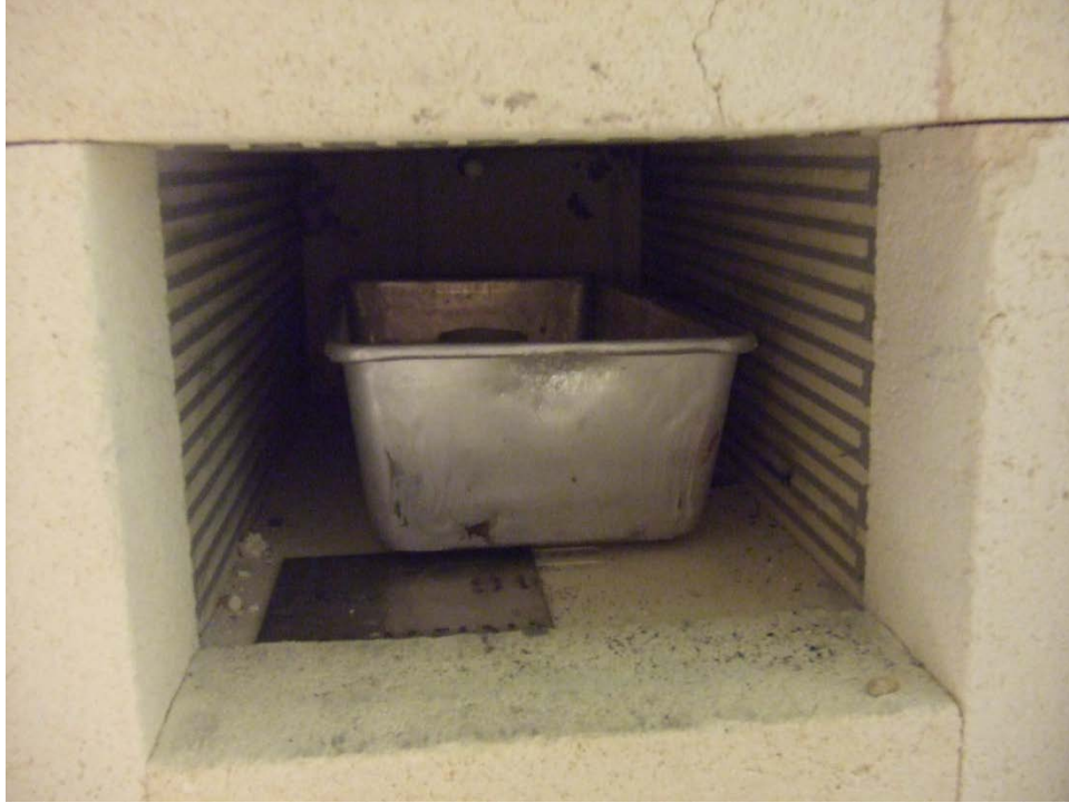
Figure 7.2.18: Oven set to 410 degrees F. Heat pipe for four minutes (with oven door closed).
