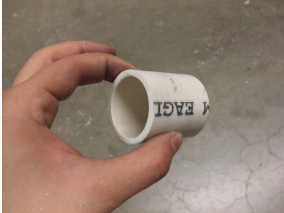
Figure 7.2.16: Short section of PVC pipe cut on band saw with fringes removed.
