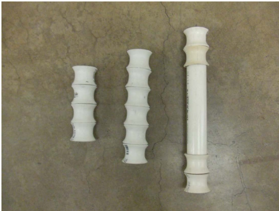
Figure 7.2.27: Three types of hinges, all are held together by a section of 1" schedule 40 pipe. A piece of 1 1/4" schedule 40 PVC pipe is used as a spacer in the largest hinge.
