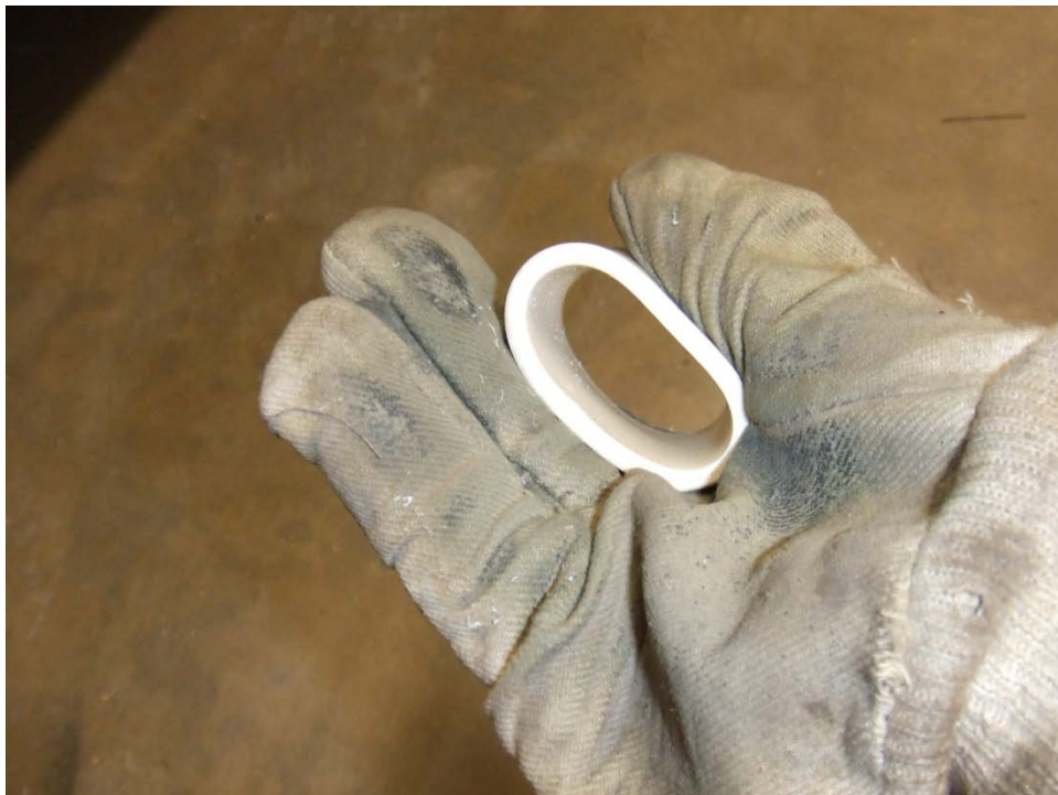
Figure 7.2.19: Heated PVC is malleable and can be formed into a variety of shapes, but still maintains most of its original structure.
