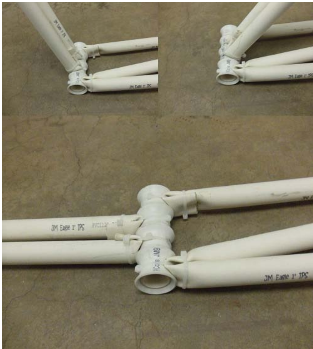
Figure 7.2.28: Rigid bodies attached to hinge with zip ties so that they are constrained to planar rotation.
