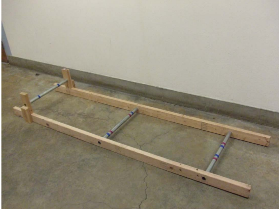
Figure 7.2.6: Jig for creating 2.97 radian displacement section and 3.08 foot sections.
