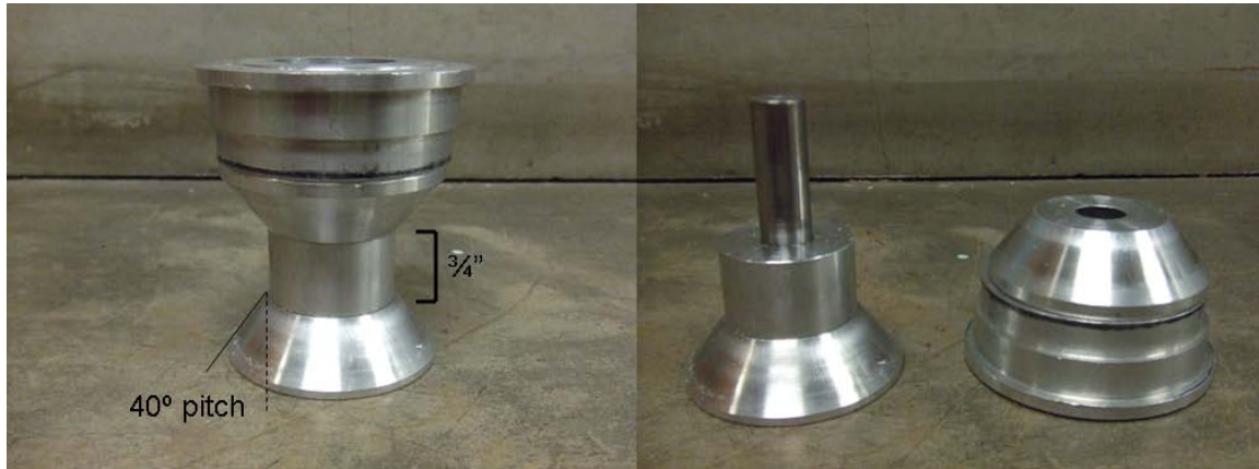
Figure 7.2.23: Hinge pressing jig with measurements and pitch indicated.
