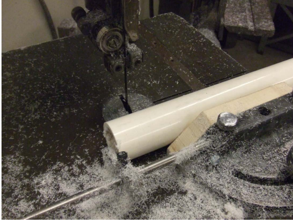
Figure 7.2.14: cutting equal 1 ½ inch segments of 1 ¼ inch schedule 40 PVC on the band saw.
