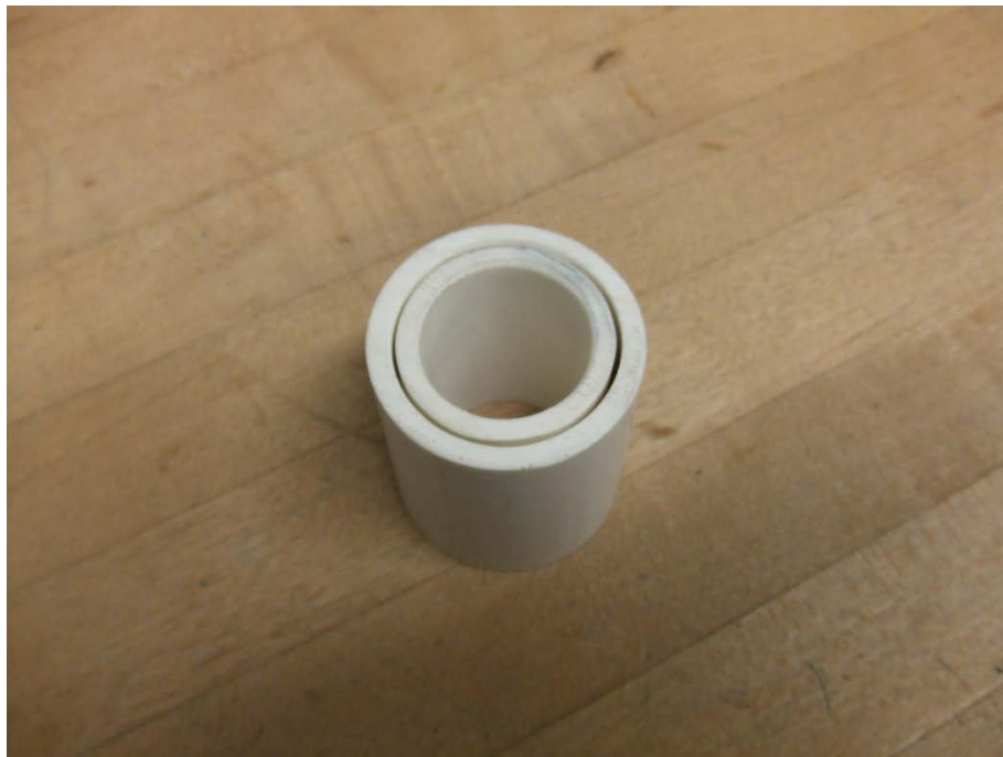
Figure 7.2.2: The 1" schedule 40 pipe fits inside the 1 1/4" schedule 40 pipe with only 1-2mm of free space. This type of fit was ideal for my hinge design (described in section 7.2.3).
